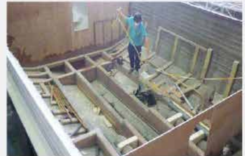
Interlocking Frames and Stringers
