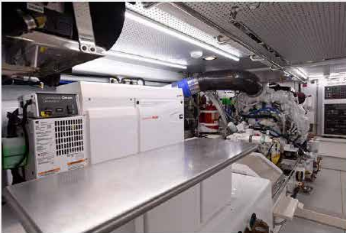
A workbench and air conditioning make the engine room a practical and comfortable workshop
